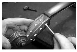
Step 9 - Apply glue to the thread Apply a small amount of polyurethane glue (eg. Selleys Urethane Bond) to the thread. Use only enough glue to fill the grooves of the thread. The use of polyurethane glue is recommended as it bonds to
