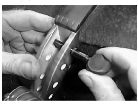
Step 11 - Clean up & let dry Wipe off any excess glue. Allow the glue to dry completely. Bed-in the action of each peg by giving it several turns while applying a gentle inwards pressure. Install the strings.
