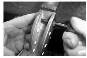
Step 3 - Mark the peg length Mark the peg where it protrudes from the peg box. Remove the peg from the peg box.
