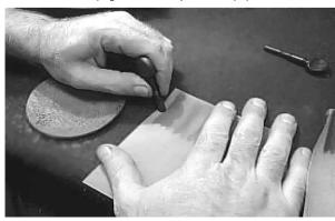
Step 7 - Shine the end Shine the peg end using the leather patch.
